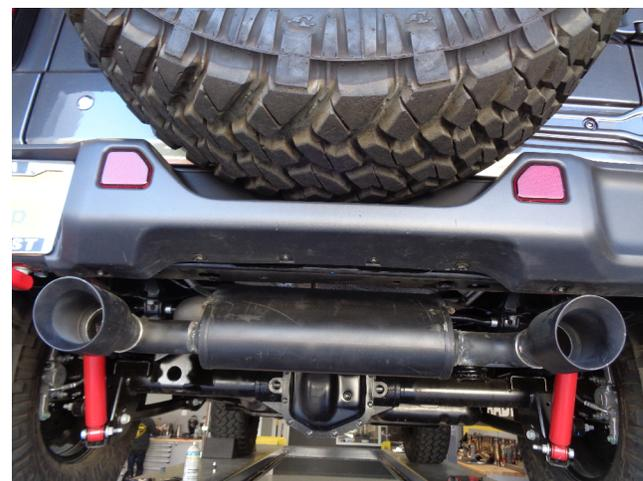
Step 3: Once a final position has been chosen for the new exhaust system, evenly tighten all clamps from front to rear using the torque specifications on page one of these instructions. Inspect all fasteners after 25-50 miles for operation and re-tighten if necessary.
