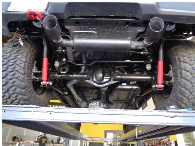
Step 2: Begin installing the new system by attaching the Muffler Assembly inlet to the OE outlet using the supplied 2.50 clamp. Engage the welded hanger to the rubber insulator. Keep all clamps and fasteners loose until final adjustment
