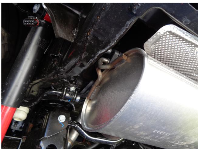
Step 1: To remove the OEM system first locate the clamp in front of the rear Muffler Assembly (located above the rear axle/sway bar) and loosen. With the Muffler supported extract the hangers from the rubber insulators and remove the muffler Assembly. Retain rubber insulators to be re-used in new installation.
